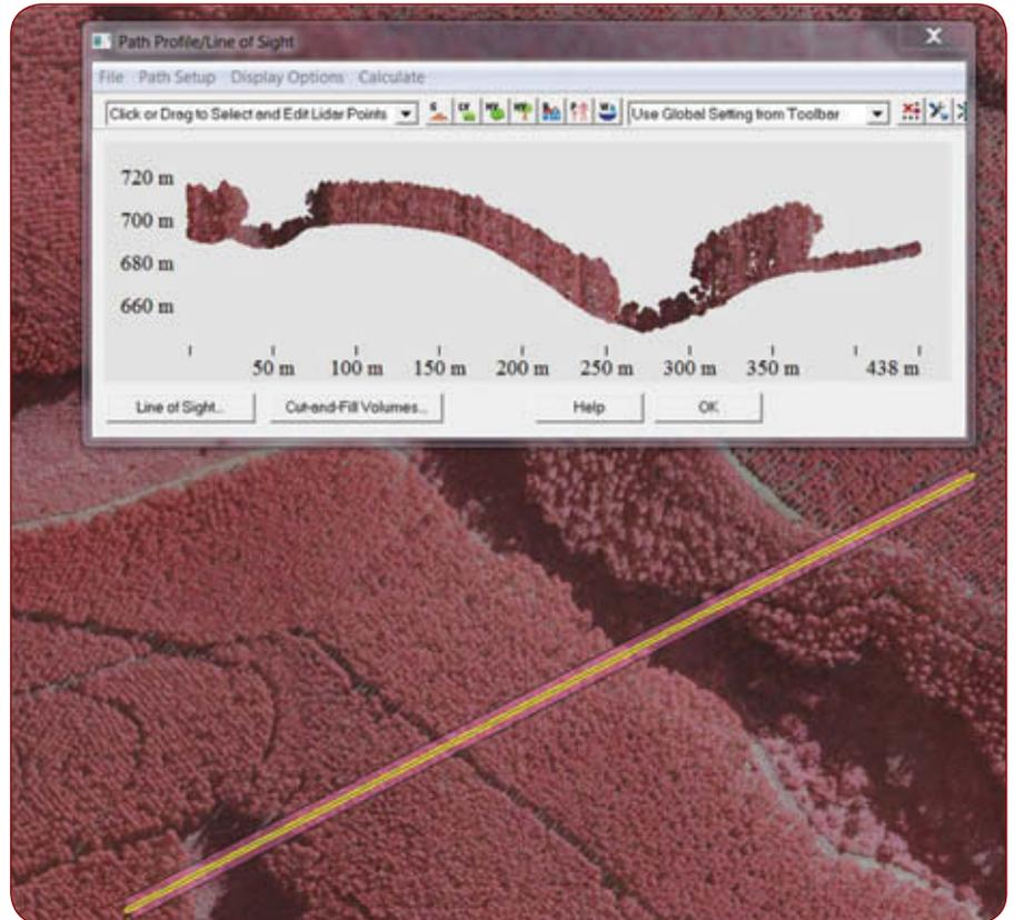
Fig. 2: Cross-sectional view of a point-cloud showing tree height in a plantation.
